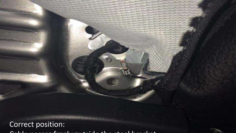
Correct position: Cable passes freely outside the steel bracket Car is OK and can be released
