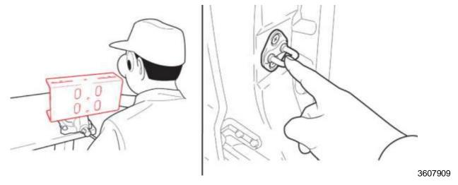
**Danger:** To avoid personal injury, *ALWAYS* keep as much of your body as possible in front of the bracket when working on the air bag assembly. Remember to periodically touch a metallic part of the vehicle or work bench to discharge static electricity in the body.
