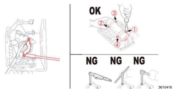
**Caution:** There will be some resistance when tightening the nuts because they are self-locking. Confirm the nuts are tightened correctly. *DO NOT* use a power tool, T-handle, or ratchet when tightening the nuts to avoid over-torqueing.
