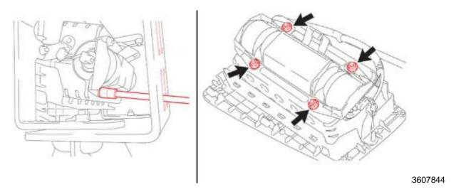
**Caution:** DO NOT use power tools. The bracket support bars may need to be repositioned to remove the nuts through the access holes.
