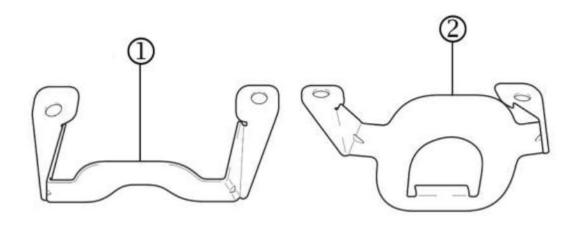
14. Confirm the identification of the stopper and the position determining plate. **THEY ARE DIFFERENT.** Refer to the illustration: (1) Stopper Plate (2) Position Determining Plate.
