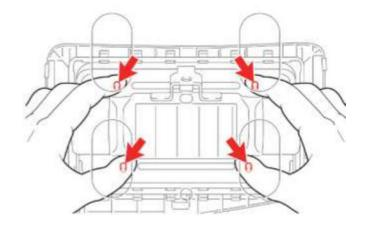
12.1 Gently push in the 4 studs to loosen the inflator for removal.
