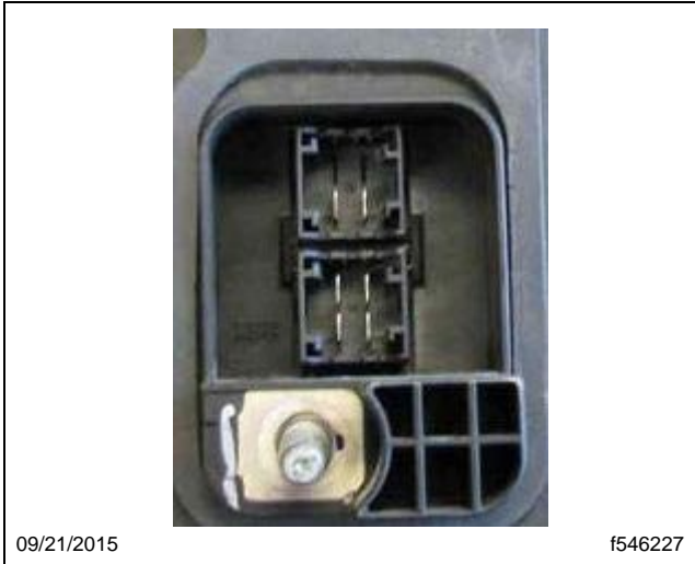
Fig. 3, Clean Terminals with No Corrosion
