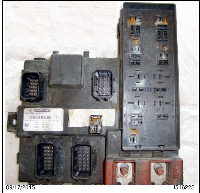
Fig. 8, Condemned SAM Chassis Photo for Warranty
