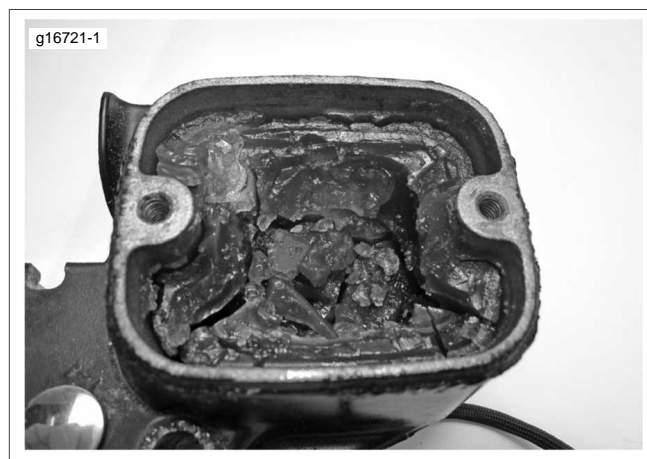
Figure 1. Fluid Gelling in Master Cylinder
