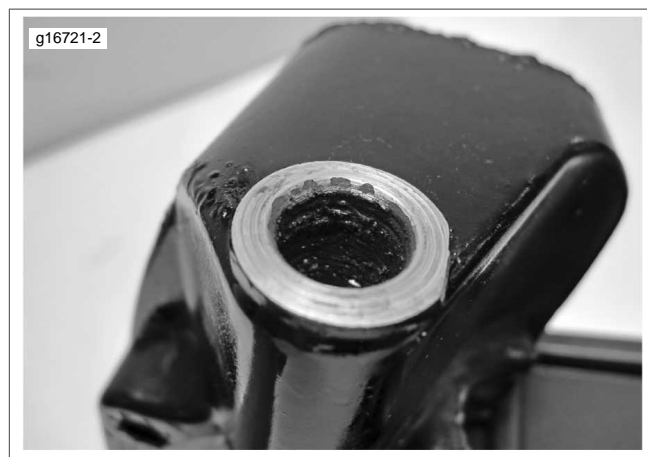
Figure 2. Banjo Bolt Hole Thread Corrosion
