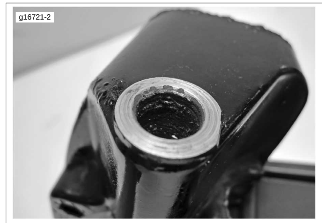
Figure 2. Banjo Bolt Hole Thread Corrosion
