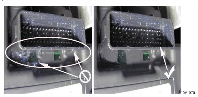
Note: Do NOT apply dielectric lubricant outside of the cavity for connector X2 (C2) in the BCM.
