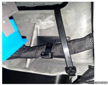
5. Install a long tie strap around the IP Mag Beam and the harness and carefully cinch the tie strap.
