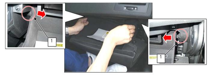
13. Remove screws (1), then remove the passenger side instrument panel undercover (2).
