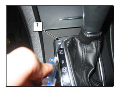
2. Push on the shift lock manual release button and shift the select lever to Neutral.
