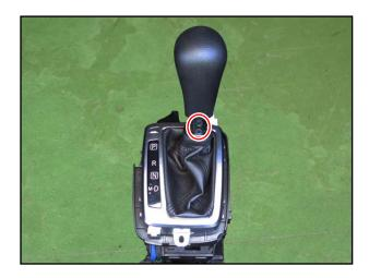
Install the select lever assembly to the floor. Torque: 13 N•m (1.3 kgf-m, 9.5 lb-ft)
