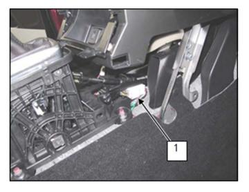
B. Detach the select cable end (1) from the select lever pin, then detach the casing cap (2) from the select lever bracket (3).
