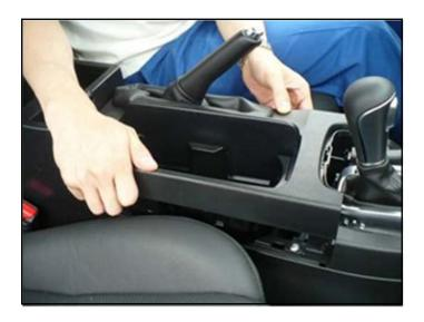
8. Pull in the direction of the arrow and remove the left and right console front garnishes (1).
