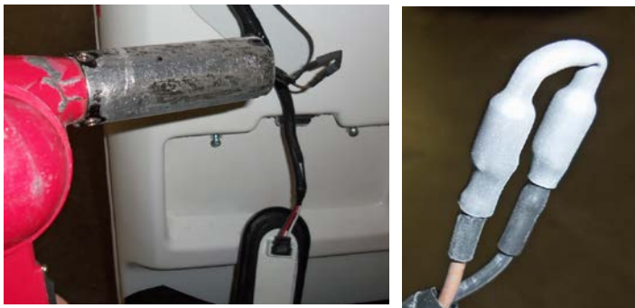
Step 3- Add a 2" piece of shrink wrap over the ends and shrink with heat gun.
