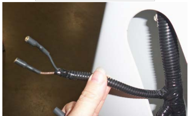
Step 2- Locate the unused side marker light connection.
