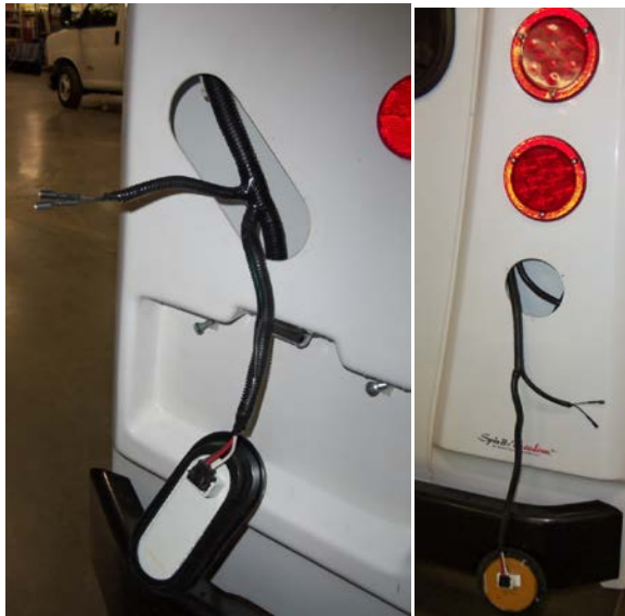
Step 3- Add a 2" piece of shrink wrap over the ends and shrink with heat gun.
