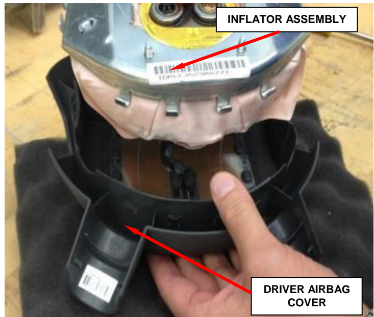
Figure 9 - Inflator Assembly to Driver Airbag Cover
