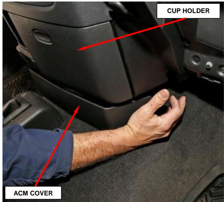
**Figure 7 – Airbag Control Module (ACM) Cover**
