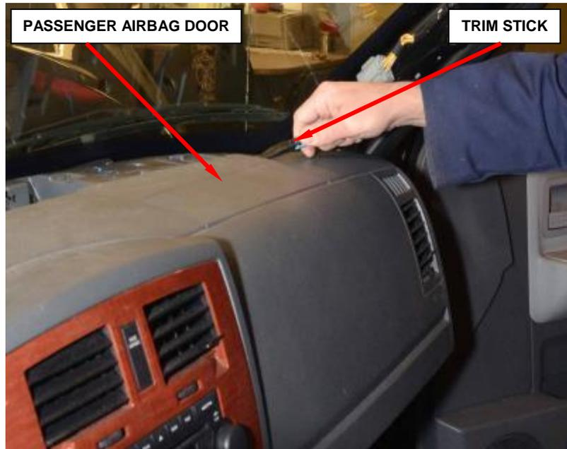
**Figure 51 – Passenger Airbag Door**
