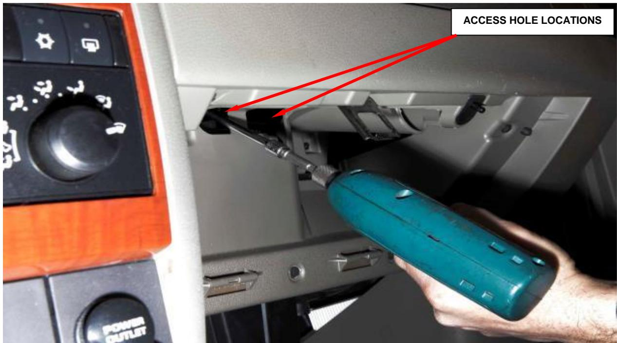
**Figure 31 - Passenger Airbag Mounting Bolt Access Holes**
