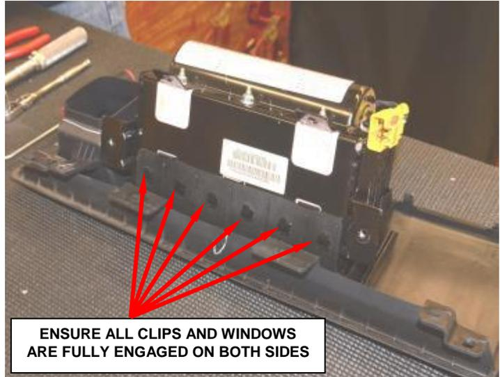
Figure 27 – Airbag Cover and Airbag Module
