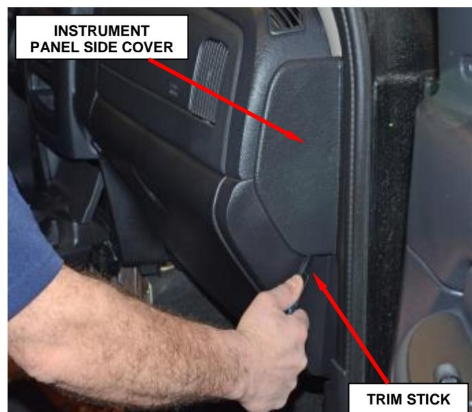
**Figure 1 – Instrument Panel Side Cover**
