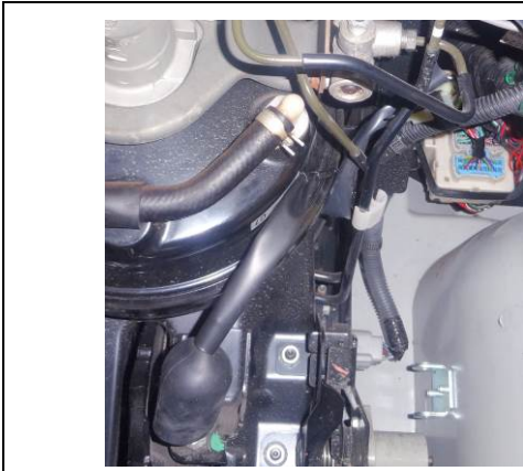
Figure 5 – Extension Harness, Installed and Secured with Band Clip
