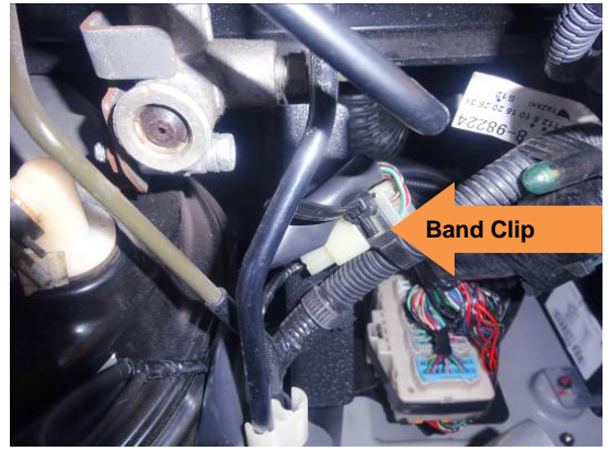
Figure 6 – Band Clip Secured to APP Sensor / Brake Stop Lamp Harness
