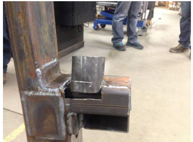
Figure 14: Proposed repair #1 after testing
