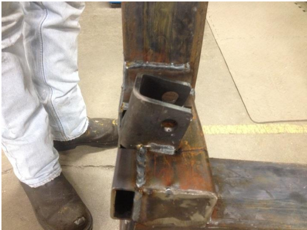
Figure 15: Proposed repair #1 after testing
