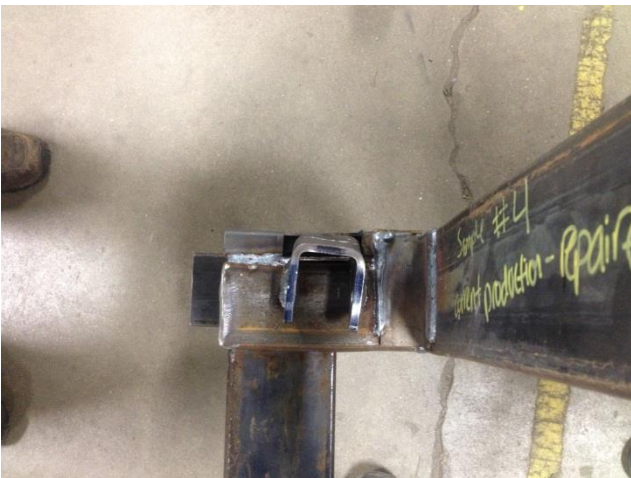
Figure 21: Proposed repair #2 after testing
