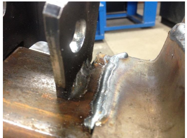
Figure 22: Proposed repair #2 after testing
