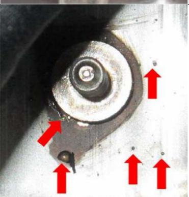
5. In some cases weld spatter might not be visible with the ground cable installed. If you encounter this situation, remove the ground cable for further inspection.
