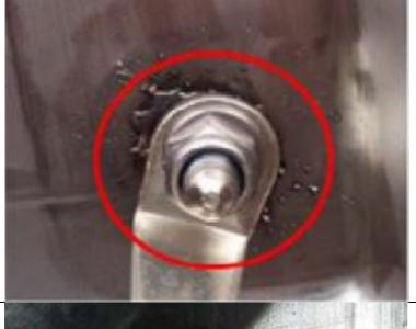
4. If weld spatter is found, the weld is leaking or the weld is questionable, Submit a standard PuMA case, with clear pictures of the weld, titled "Recall Campaign 14V-674: I12 Check Fuel Tank."
