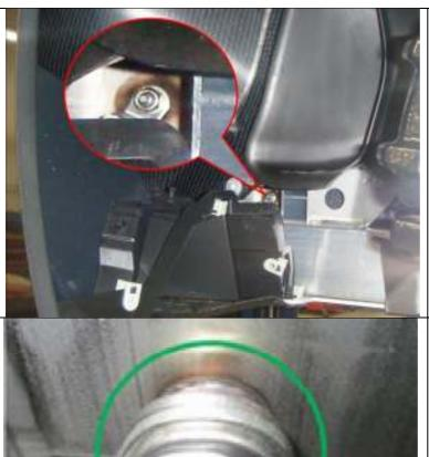
2. Visually inspect the weld of the fuel tank ground stud through the wheel arch.
