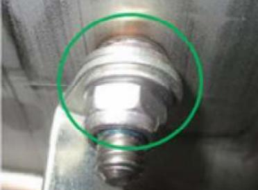
3. If the weld is clean and free of weld spatter and is not leaking, no further steps are required and the vehicle can be delivered to the customer.
