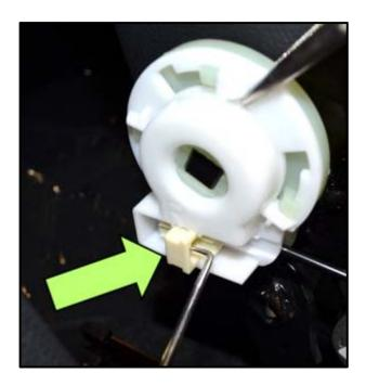
Use a 90° pick tool (or equivalent) to partially remove the clip <arrow>.
