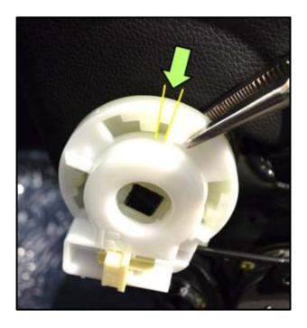
← If a gap is present between the locking ears of the rotating plate, and the hard stop on the ground plate as shown <arrow>, release the locking pliers, turn the rotating plate in the appropriate direction to close the gap completely, then reattach the locking pliers.
