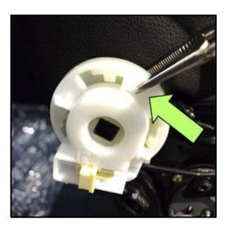
Lightly clamp a pair of needle nosed locking pliers (or equivalent) onto the outboard seat recliner mechanism as shown <arrow>.
