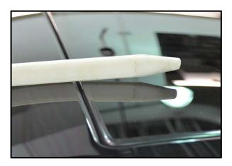
Note: When adjusted correctly, the front edge of the sunroof glass should be roughly 1mm below the roof of the vehicle, and the rear edge of the sunroof glass should be roughly 1mm above the roof of the vehicle.
