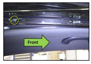
Remove the rear corner mounting screw <circle> from the left and right sides.
