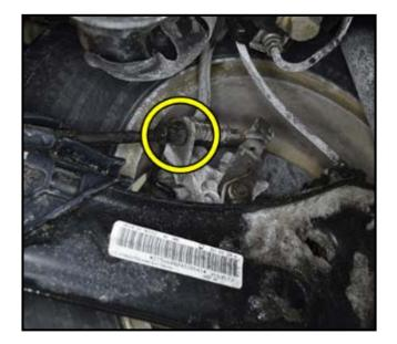
⇐ Disengage the parking brake cable <1> from the mounting hook <2> and pull it from the guide tube <3>.
