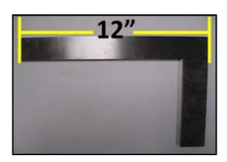
Tip: Example of equivalent tool: Carpenter square measuring 12 inches (~300mm) in length.
