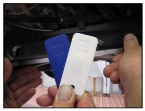
Hold the blue (1.25mm thickness) and the white (1.0mm thickness) gauges together to achieve a 2.25mm measurement.
