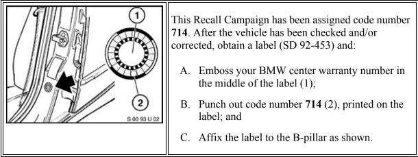
If the vehicle already has a label from a previous Service Action/Recall Campaign, affix the new label next to the old one. Do not affix one label on top of another one because a number from an underlying label could appear in the punched-out hole of the new label.
