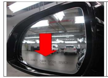
If Korean text is seen on the mirror, it must be replaced with the correct US version.
