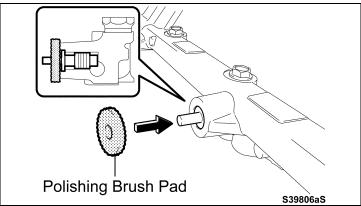
h) Place the NEW polishing pad onto the guide in the fuel delivery pipe.
