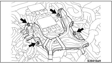
I) Remove the 4 nuts and remove the lower cover.
