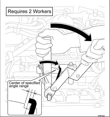
i) Tighten the sensor until the needle tip aligns with the center of the cut out in the plate as shown.
