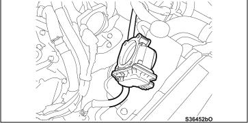
e) Place the throttle body on the reservor tank.
