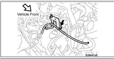
g) Reinstall the bracket and bolt Torque: 10 Nm (102 kpf-cm, 7 ft-lbs)
