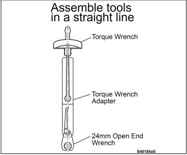
f) Assemble the 24 mm wrench, torque adapter and the supplied torque wrench as shown.
