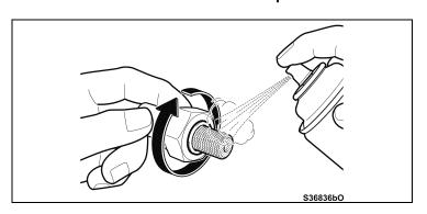
d) Spray Pando 39C onto the threaded portion of the sensor.
