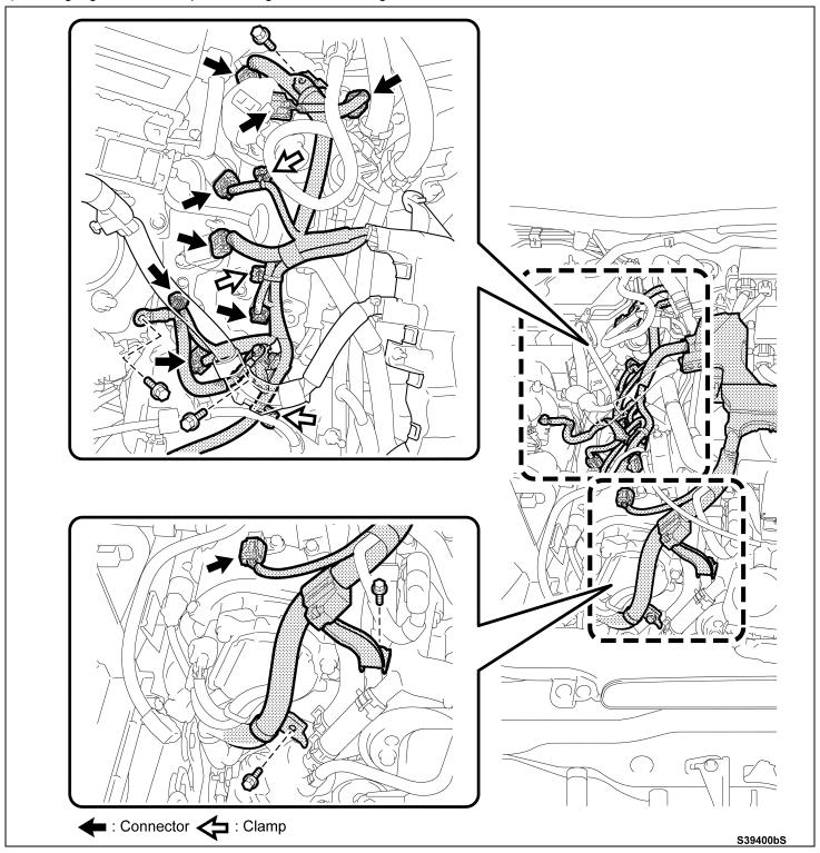
g) Remove the 2 bolts bolts and disconnect the connectors.
