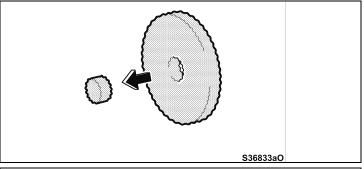
f) Inspect the polishing pad that is contained in the parts kit. Ensure that the center piece of the new pad is removed.
