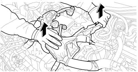
2. The main worker must temporarily install the manifold while the assisting worker is lifting the wire harnesses, avoiding damage to the injectors due to interference with other parts. (Work from the left side of the vehicle)
