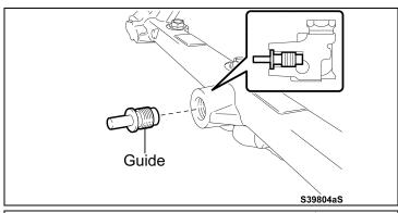
e) Install the guide into the fuel delivery pipe finger tight.
