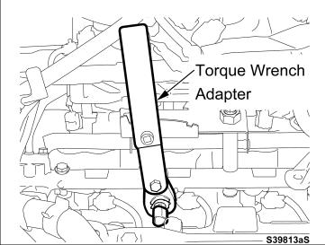
e) Place the 24 mm wrench onto the sensor with the needle as close as possible to the zero position of the torque plate.
