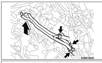
j) Release the 3 clips and remove the 3 hoses while lifting the pipe at an angle.
