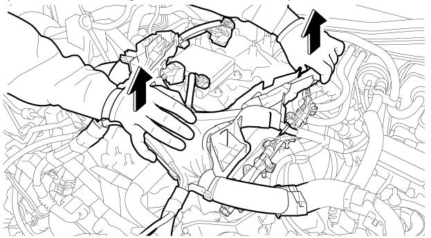
2. The main worker must remove the No. 2 delivery pipe while avoiding damage to the injectors by interference with other parts. (Work from the left side of the vehicle)
