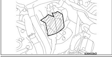
g) Place protective tape over the throttle body opening to prevent foreign objects from entering the surge tank.
