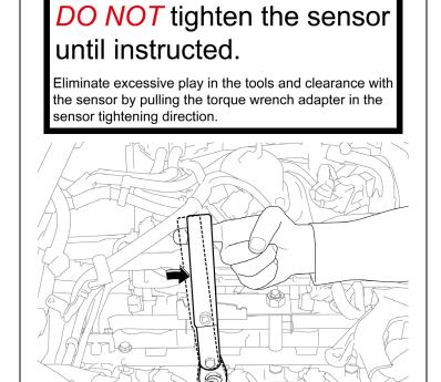
g) Lightly push and hold the torque adapter as shown to eliminate any play but do not rotate the sensor.
