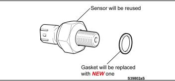
e) Remove the tool from the sensor and remove the sensor by hand.
