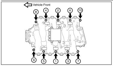
e) Reinstall the 8 bolts and the 2 nuts in the sequence shown.
