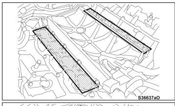
j) Cover the openings with tape to prevent foreign objects from entering the intake ports.
