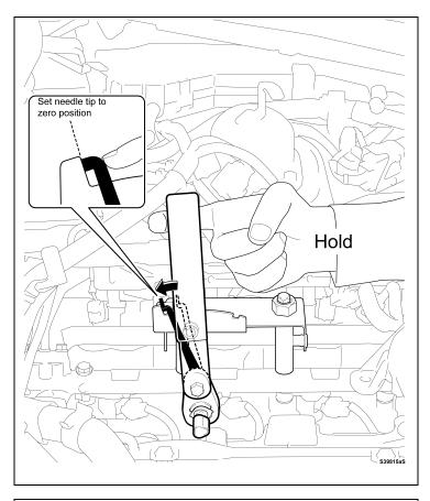
h) While holding the torque adaptor gently move the needle on the 24 mm wrench to the zero position on the plate.
