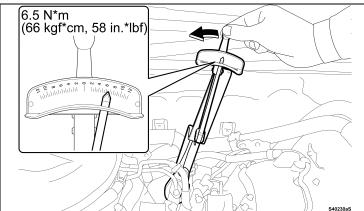
g) Tighten the sensor as shown until the specified torque reading is obtained.
