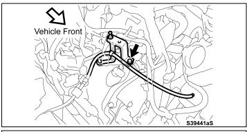
e) Remove the bolt from the bracket and move the bracket to provide clearance to remove the surge tank.
