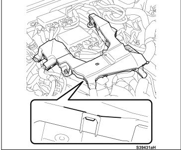
j) Disengage the 30 claws around the edge of the No. 4 harness upper cover.
