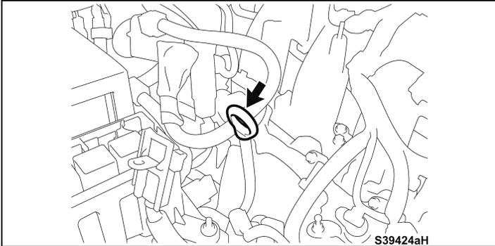
d) Remove the engine dip stick.
