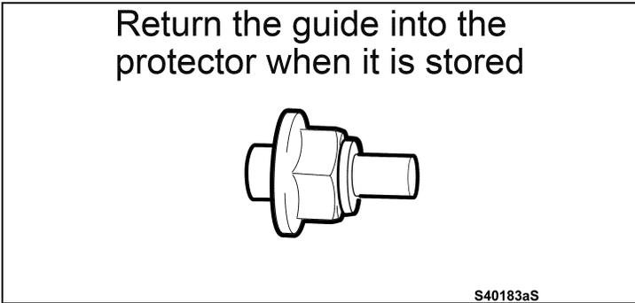
p) Reinstall the guide into the protector to protect the threads.
