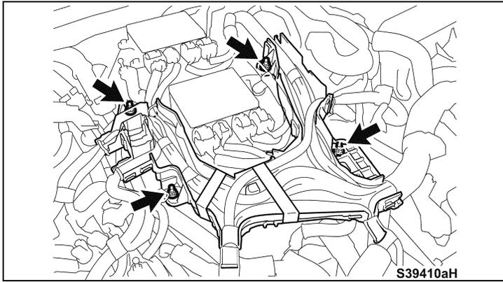
l) Remove the 4 nuts and remove the lower cover.
