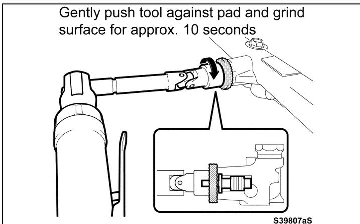
k) Gently push the tool and pad against the end of the delivery pipe.
