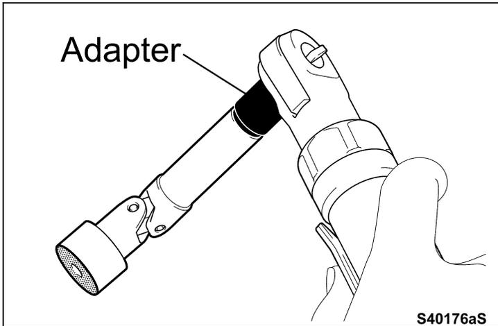
i) Check that the air ratchet will rotate clockwise.
