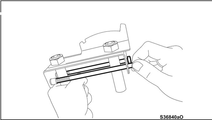
b) Remove the 2 bolts from the supplied UR torque angle plate.
