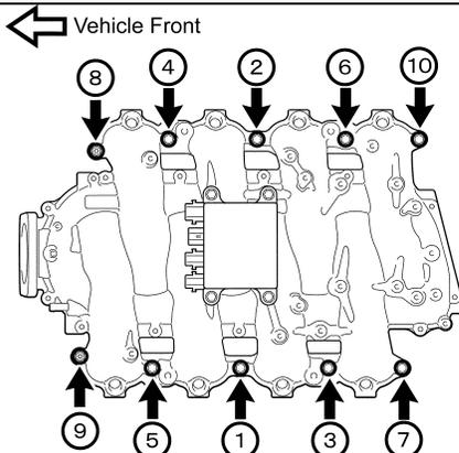
e) Reinstall the 8 bolts and the 2 nuts in the sequence shown.
