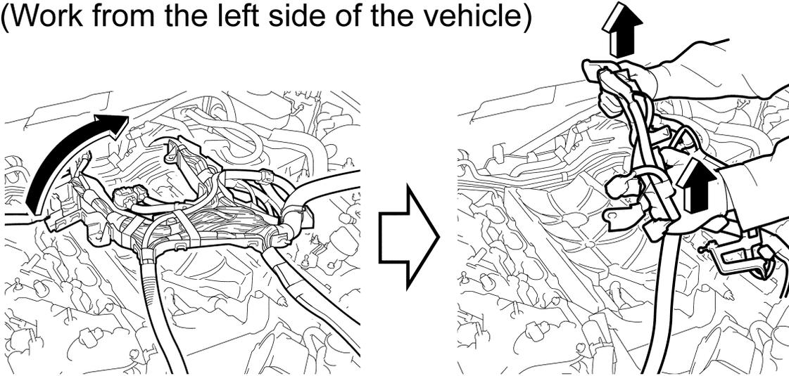
2. The main worker must temporarily install the surge tank while the assisting worker is lifting the wire harness.
