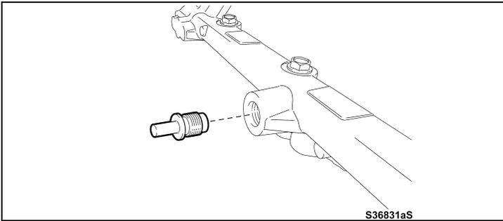
o) Remove the guide from the end of the pipe.
