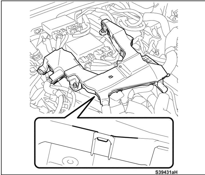
j) Disengage the 30 claws around the edge of the No. 4 harness upper cover.
