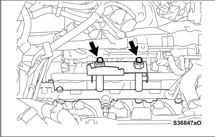
k) Remove the 2 bolts shown and remove the plate.
