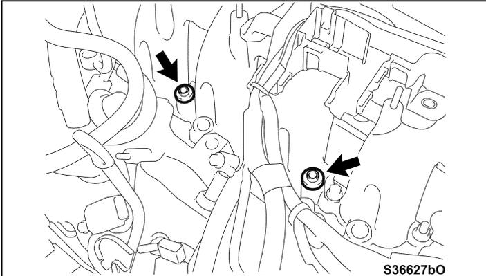
c) Remove the 2 No. 1 delivery pipe spacers.
