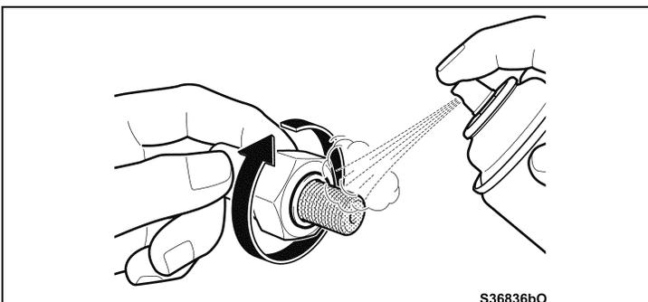
d) Spray Pando 39C onto the threaded portion of the sensor.
