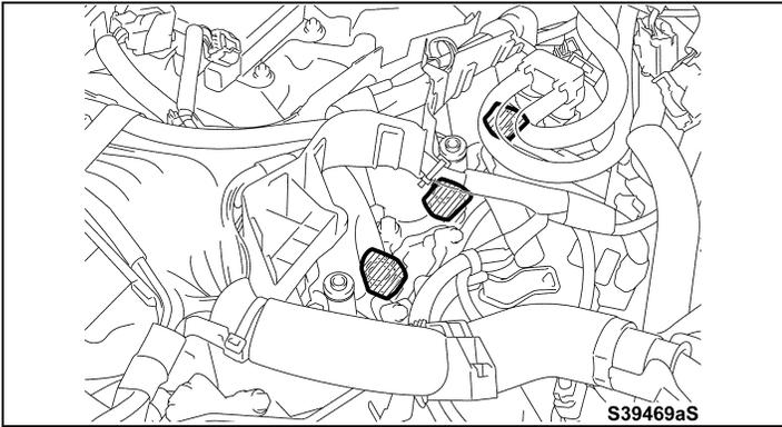
d) Cover the injector port openings with tape.
