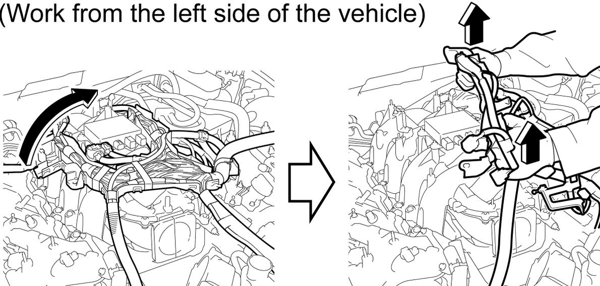
2. The main worker must remove the intake air surge tank while the assisting worker is lifting the wire harnesses. (Work from the right side of the vehicle)
