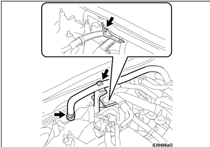
i) Reinstall the bolt onto the wire harness bracket.
