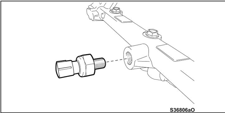
e) Reinstall the sensor into the pipe.
