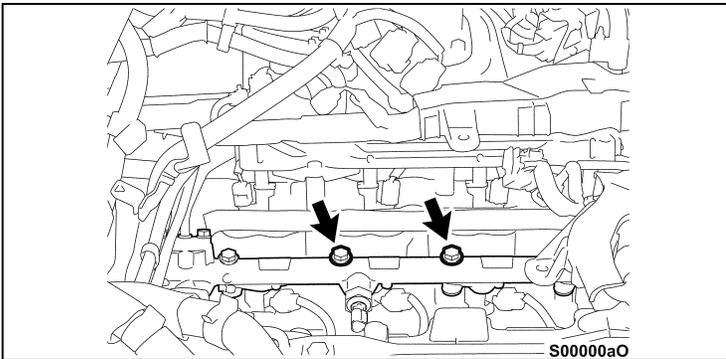
m) Reinstall the bolt and nut for the right fuel delivery pipe.
