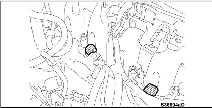
b) Cover the injector port openings with tape.
