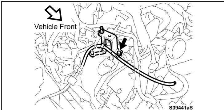
g) Reinstall the bracket and bolt
