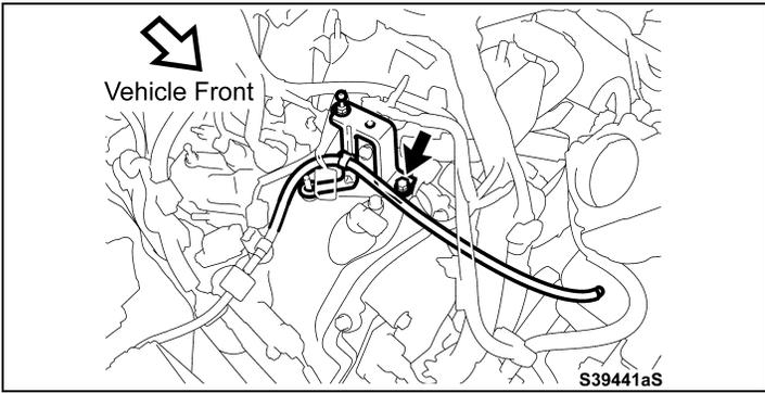
e) Remove the bolt from the bracket and move the bracket to provide clearance to remove the surge tank.
