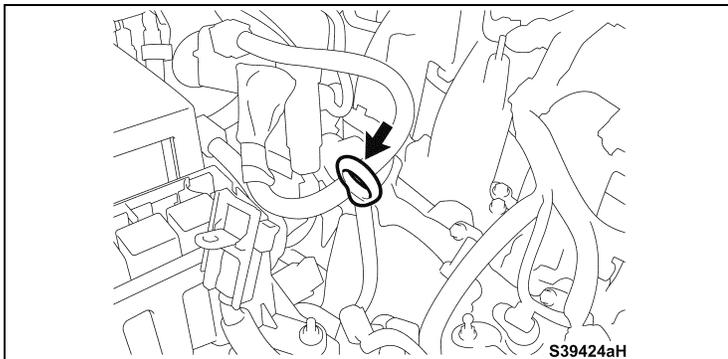
h) Reinstall the engine dip stick.
