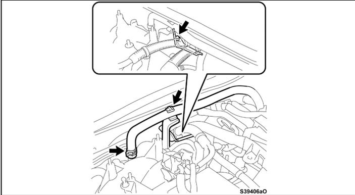
b) Disengage the clip and separate the vacuum hose.
