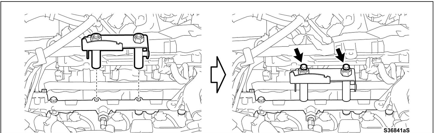
**DO NOT skip the torque angle procedure it is the critical step in this repair.**
