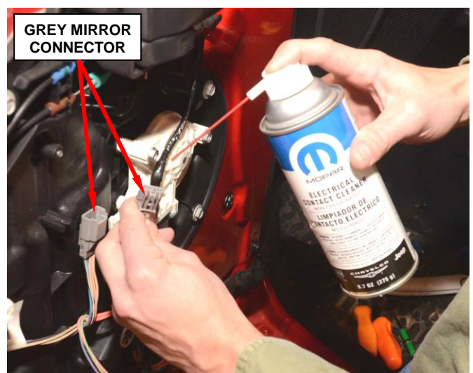
Figure 3 – Clean Electrical Connectors
