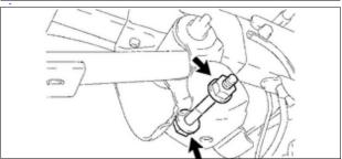
Align the holes and install the NEW hardware (bolt, washer and nut).
