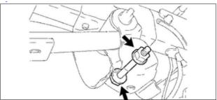
b) Align the holes and install the *NEW* hardware (bolt , washer and nut).
