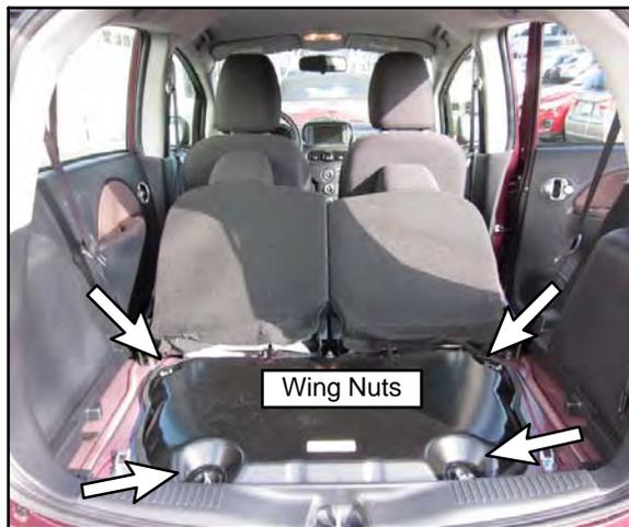
3. Open the liftgate. Fold the rear seatbacks forward into the passenger compartment.
