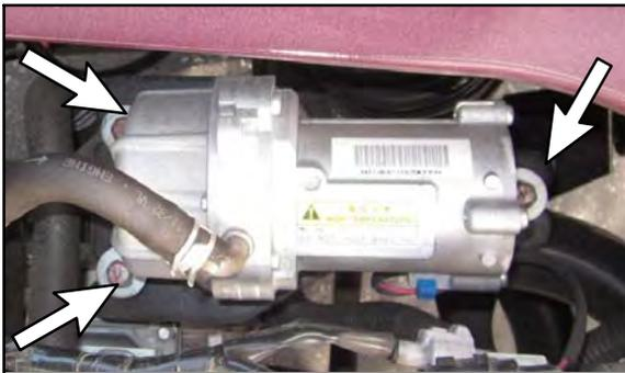
11. Remove three 12mm bolts to disconnect the vacuum pump assembly.
