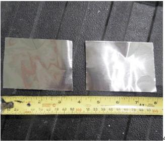
47.1 Cut the heat tape in half. Each piece of tape will be approximately 89 mm (3.5 in) long.
