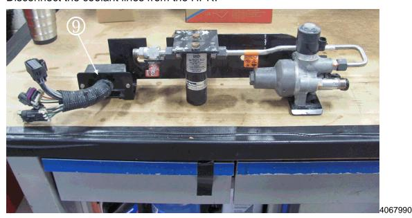
CNG control module (9) installed on the new regulator and bracket assembly.
