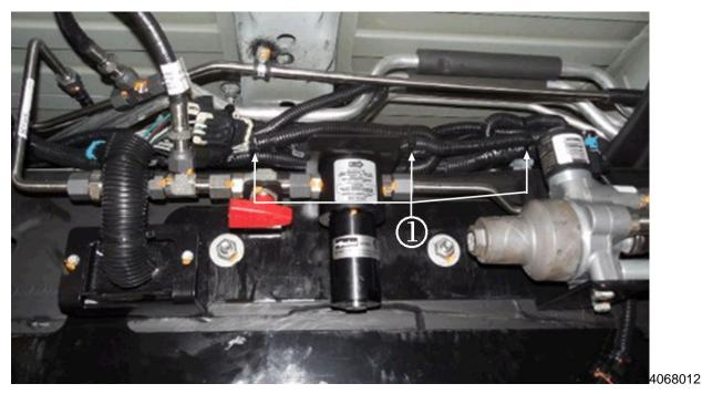
**Note:** Cut and remove the tie straps at the harness connections. Take a picture of the harness routing and tie strap location points (1) to aid in the routing and installation of the harness in step 37. One tie strap is located just to the right of all the connectors and just to the left of the ¼ turn valve. The second tie strap is located just to the right of the filter and the third tie strap is above the regulator.
