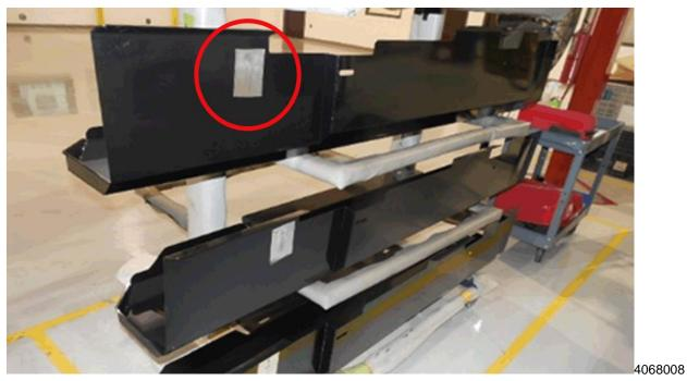
47.3 Peel and discard the heat tape backing material and apply one half of the cut heat tape over the same PRD vent opening on the outside of the mid ship tank shield as shown. Make sure the tape is centered and covers the opening completely.
