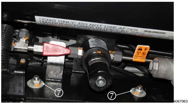
New regulator and bracket assembly shown. Production regulator and bracket are similar.
