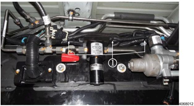
**Note:** Secure the harness connectors with a tie strap. Bundle the rest of the harness on top of the chassis rail. Secure the harness to the rear chassis harness with two additional tie straps. Install one tie strap to the right of all the connectors and just to the left of the ¼ turn valve. Install the second tie strap to the right of the filter. Install the third tie strap above the regulator.
