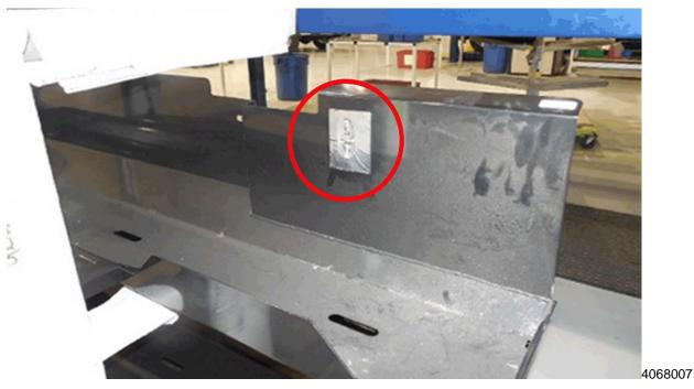
47.2 Peel and discard the heat tape backing material and apply one half of the cut heat tape over the PRD vent opening on the inside of the mid ship tank shield as shown. Make sure the tape is centered and covers the opening.
