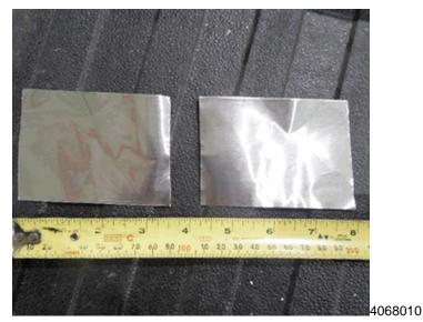
47.1 Cut the heat tape in half. Each piece of tape will be approximately 89 mm (3.5 in) long.
