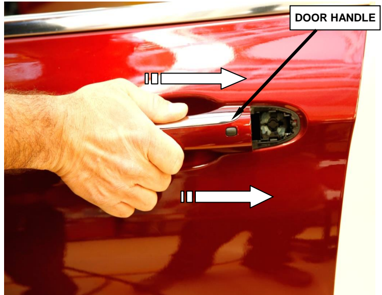
Figure 9 – Door Handle Removal
