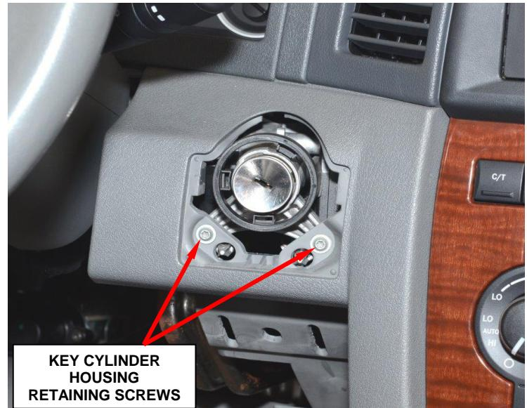
**Figure 3 – Key Cylinder Housing Retaining Screws**
