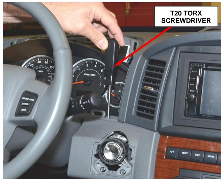
**Figure 6 – Third Key Cylinder Retaining Screw Location**
