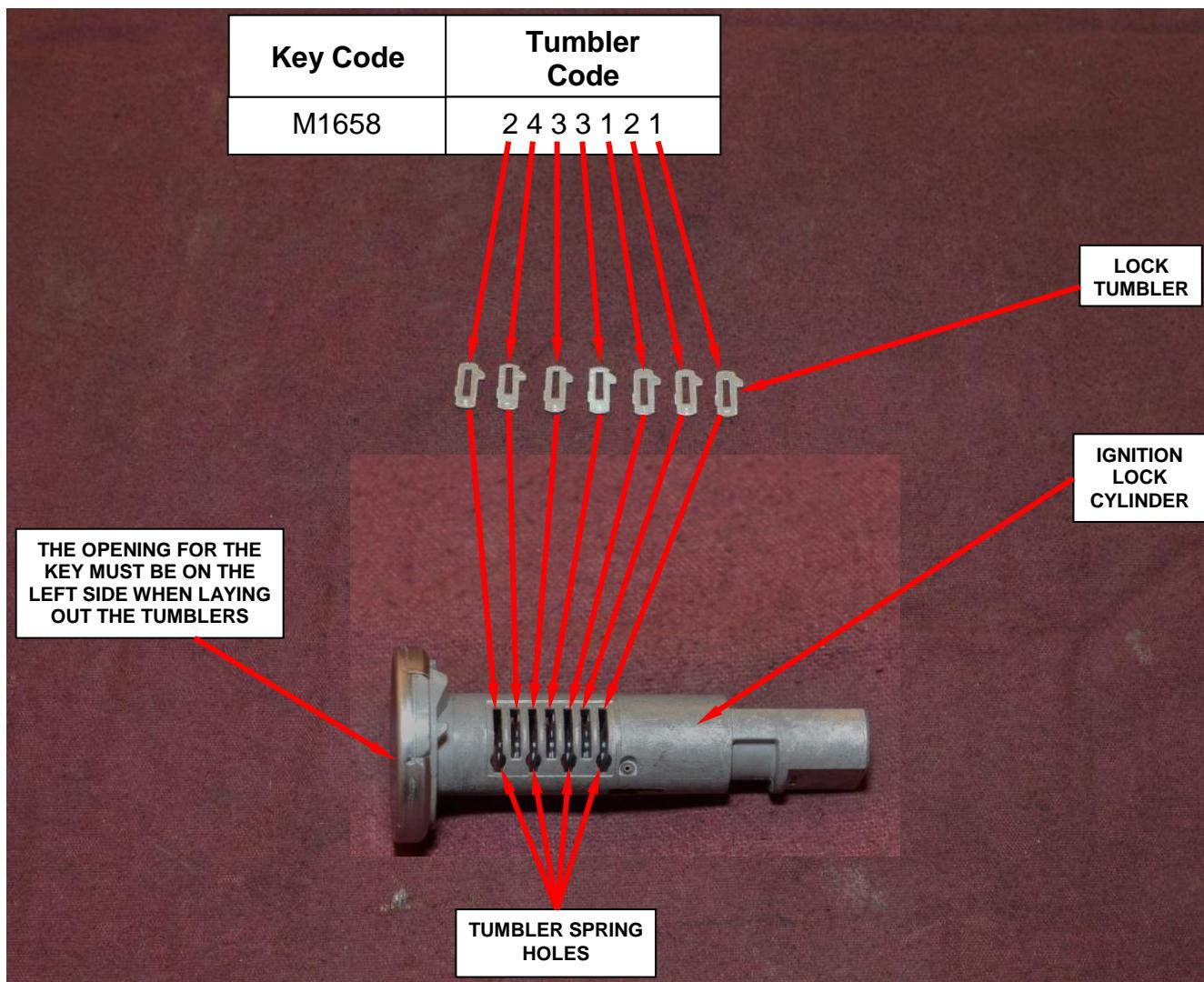
**Figure 12 – Determining Correct Tumblers and Locations**
