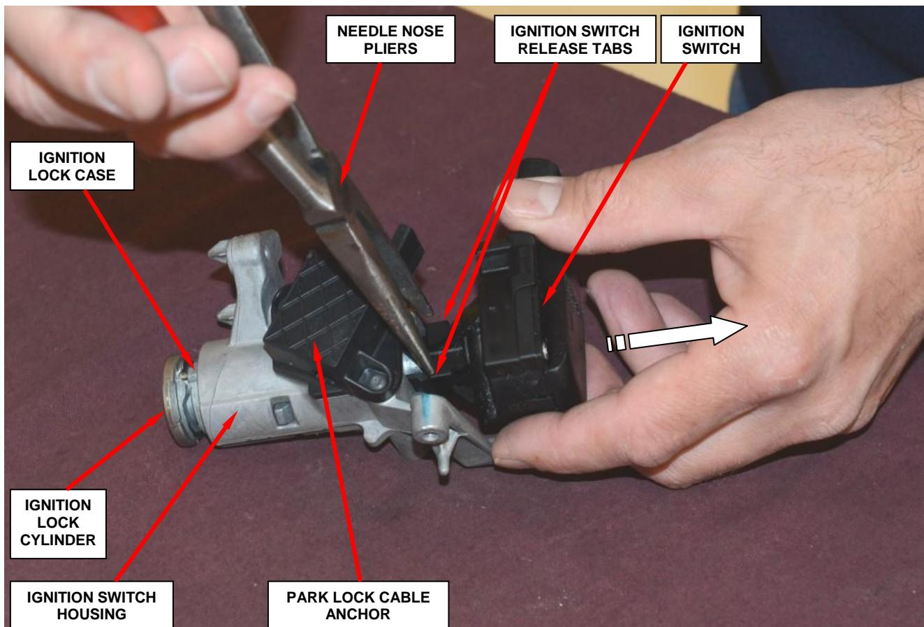
Figure 10 – Ignition Switch Removal
