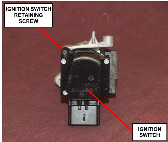
13. Using needle nose pliers, simultaneously press in the two ignition switch release tabs and remove the original ignition switch by pulling the ignition switch from the ignition switch housing (Figure 10).
