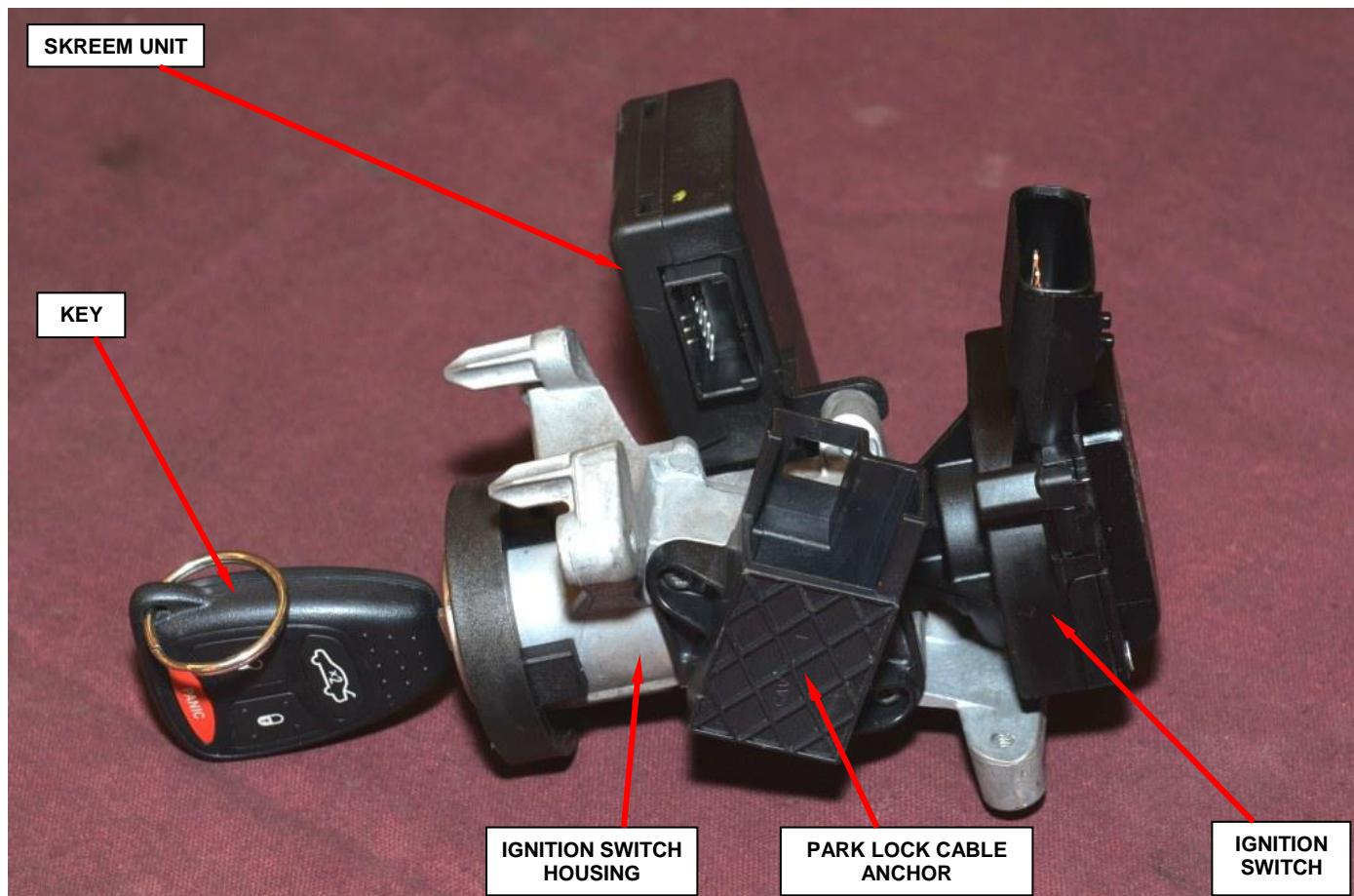
**Figure 8 – Ignition Key Cylinder Assembly**
