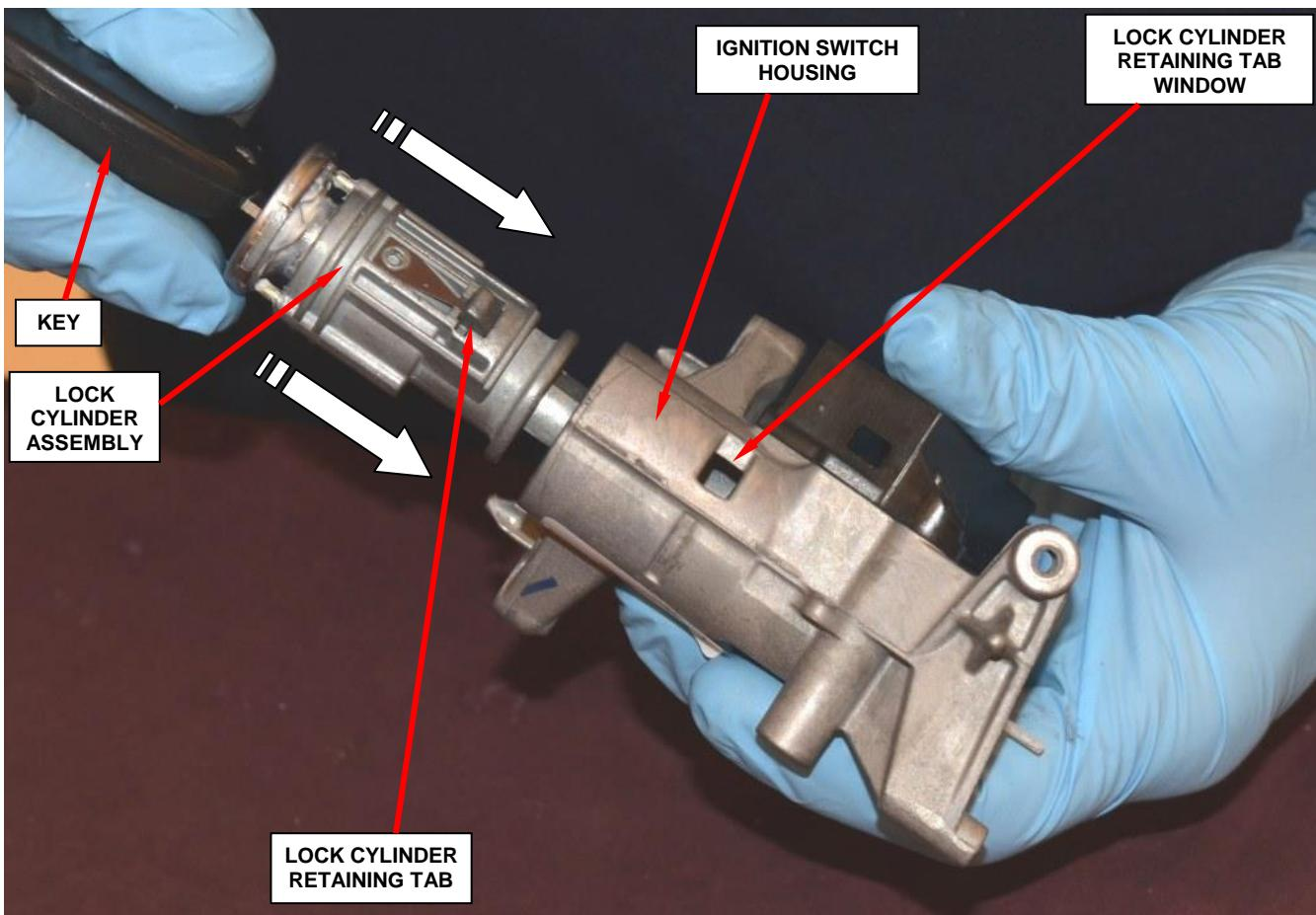
**Figure 18 – Insert Key Lock Cylinder into Lock Housing**
