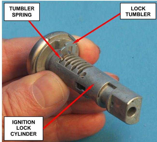
**Figure 13 – Tumbler and Spring Installation**
