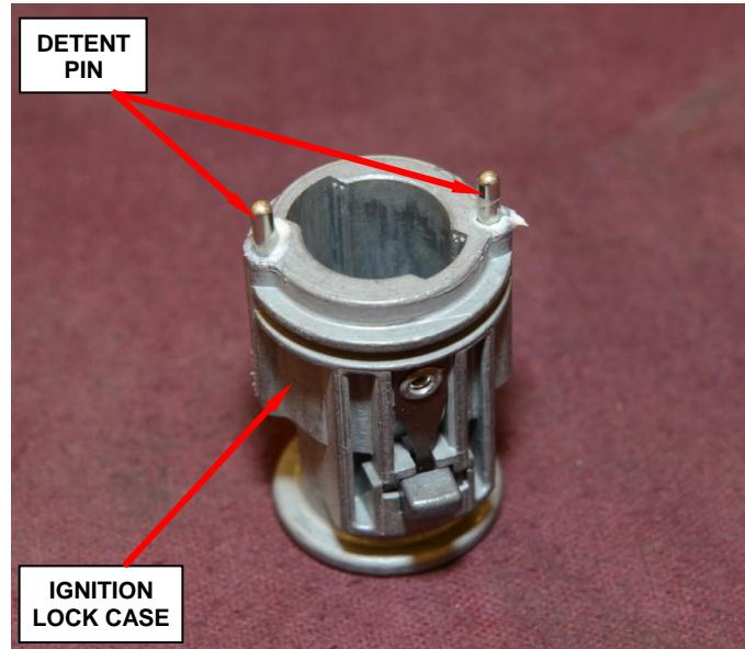
21. Apply grease to the detent springs and detent pins (Figure 15).
