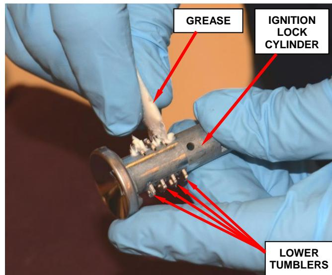
**Figure 16 – Grease Tumblers and Ignition Lock Cylinder**
