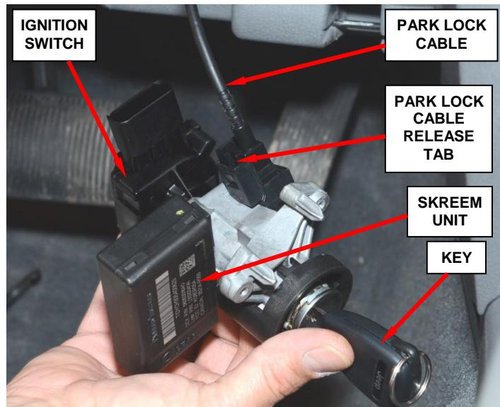
**Figure 7 – Park Lock Cable Release Tab**
