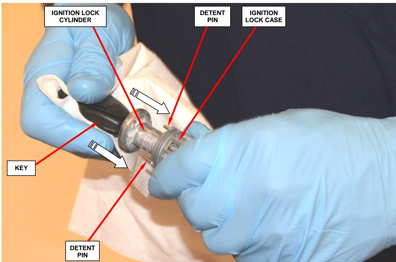
**Figure 17 – Insert Ignition Lock Cylinder into the Ignition Lock Case**
