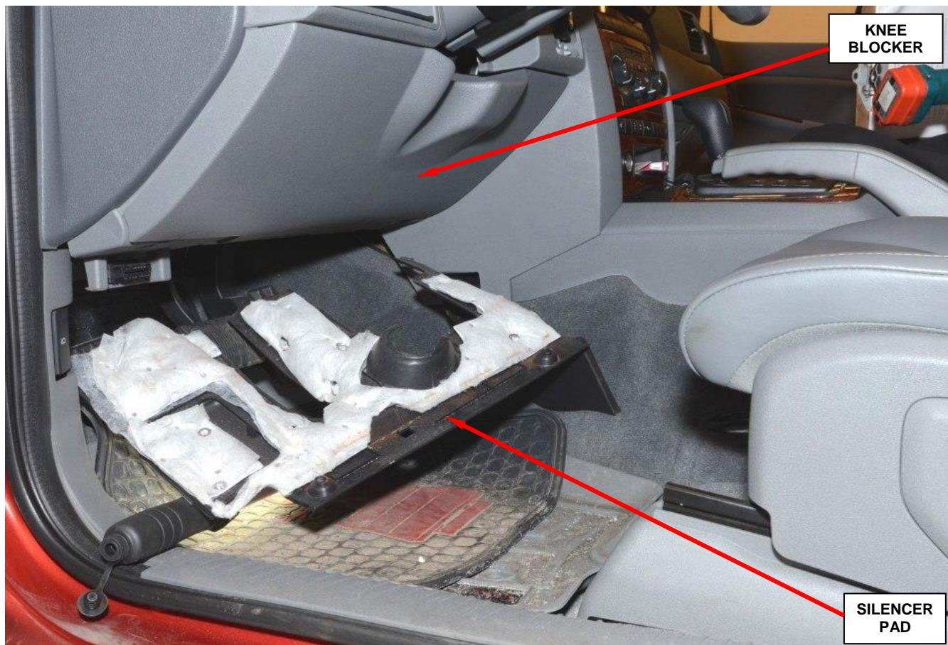
**Figure 2 – Silencer Pad and Knee Blocker**
