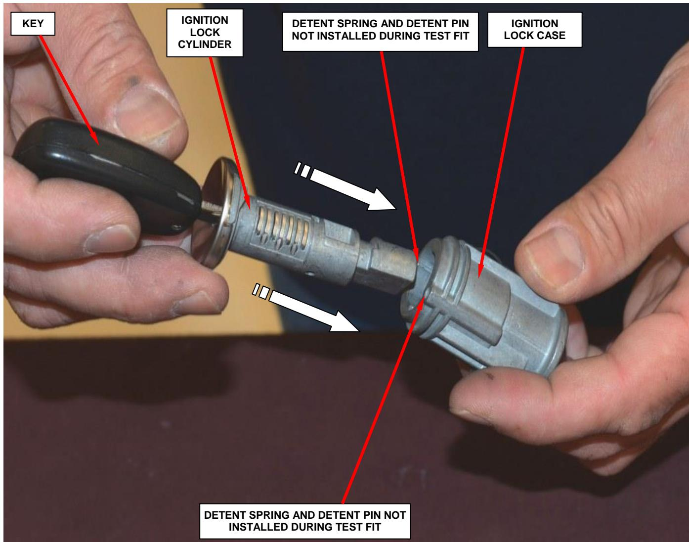
**Figure 14 – Insert Ignition lock cylinder into Lock Cylinder (without Detent Springs and Pins) and Check for Binding**
