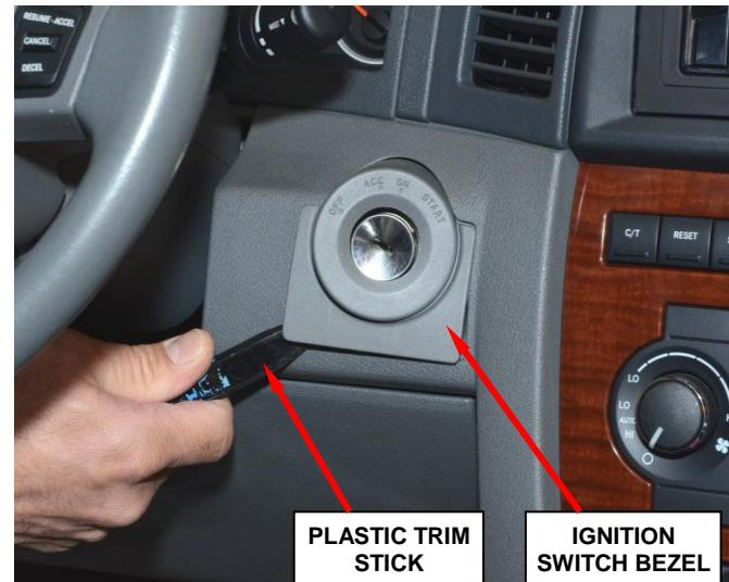
**Figure 1 – Ignition Switch Bezel**
