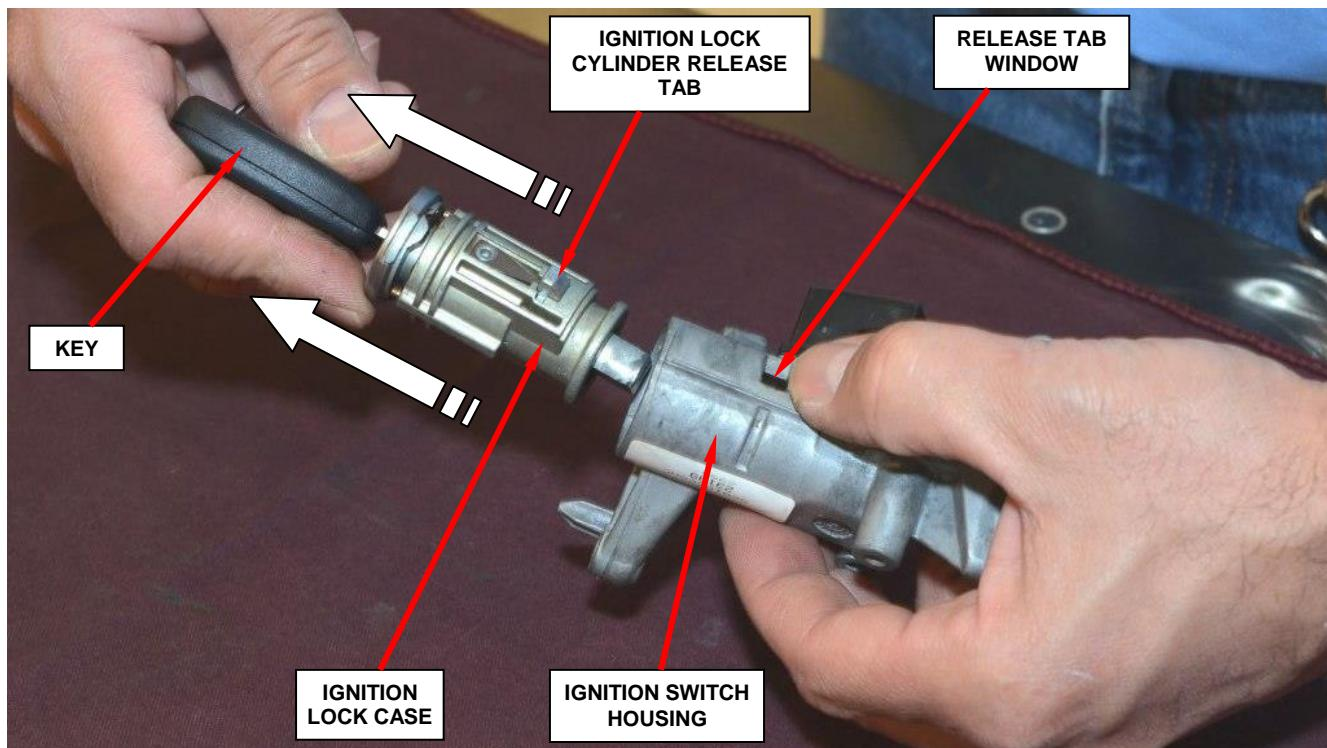
**Figure 11 – Remove Original Key Lock Cylinder from Ignition Switch Housing**
