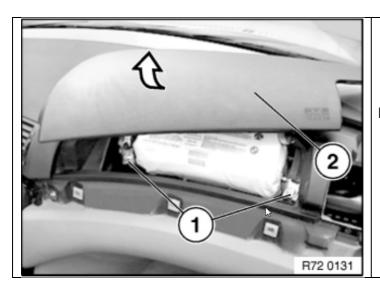
Undo the screws (1) and place the front passenger's airbag cover (2) on top.
