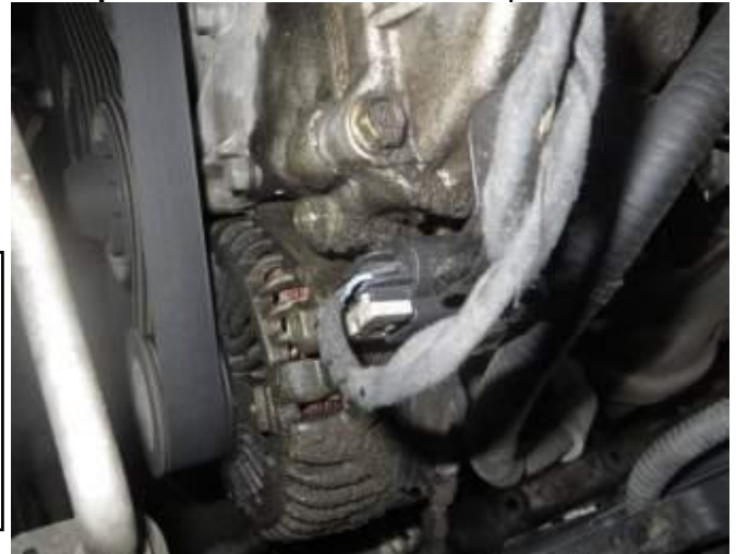
Example: Oil Contamination → Replace Alternator
