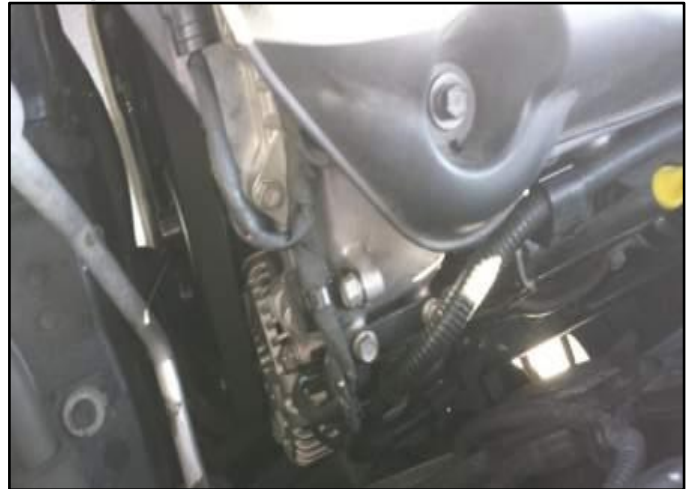
Example: No Oil Contamination → Good Alternator
