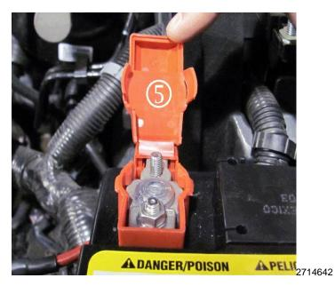
12. Open the battery positive terminal cover (5) on the auxiliary battery.
