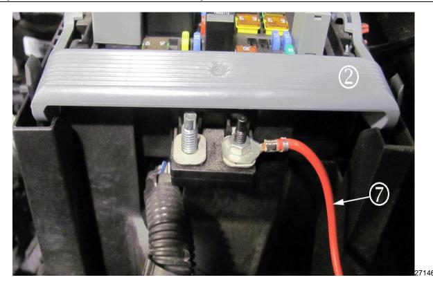
16. Press down on the underhood electrical center/junction block retainer (2) to secure the underhood electrical center/ junction block to the bracket.
