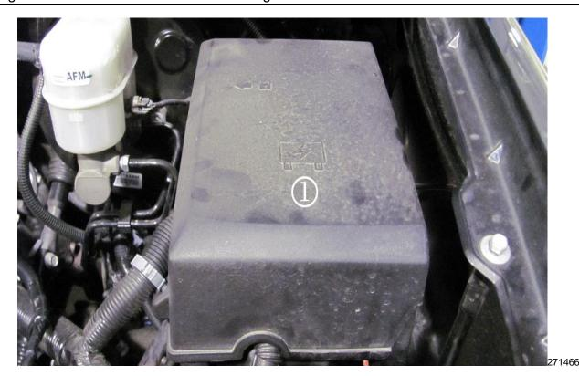
3. Remove underhood electrical center/junction block cover (1). Refer to *Underhood Electrical Center or Junction Block Replacement* in SI.
