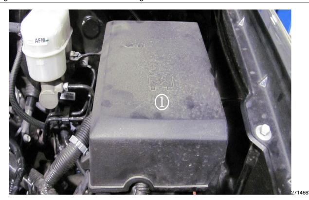
18. Install underhood electrical center/ junction block cover (1). Refer to *Underhood Electrical Center or Junction Block Replacement* in SI.
