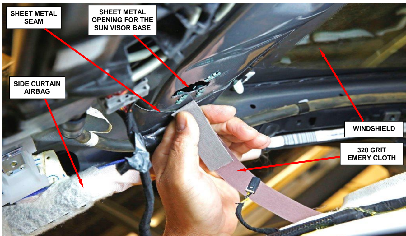
Figure 11 – Dull Sheet Metal Seam Edge (right side shown)
