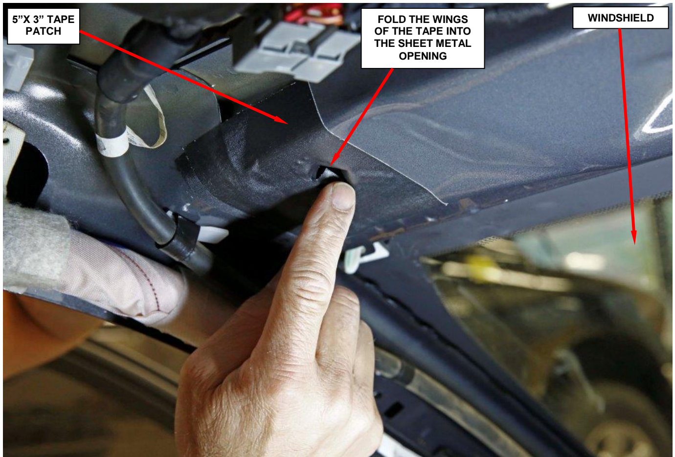
Figure 17 – Fold Tape Wings into the Hole
