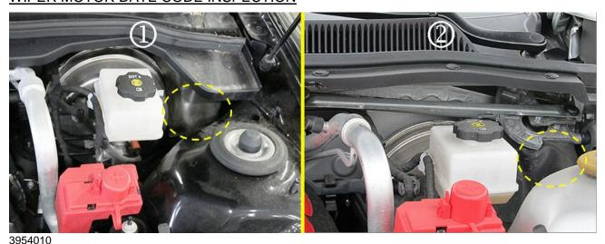
**NOTE**: Examples of the wiper motor water shield locations for Caprice PPV (1) and Chevrolet SS (2) are shown in the graphic above.
