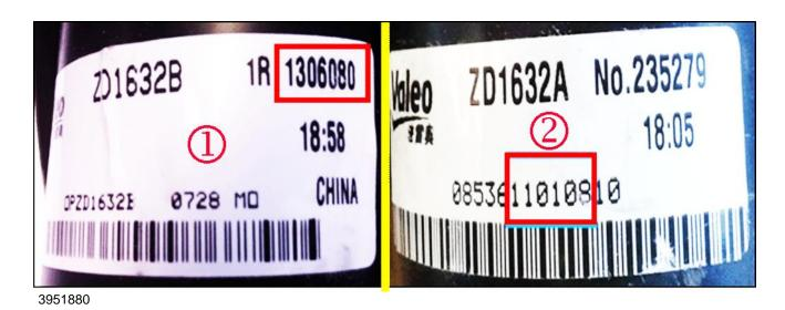
**Example (1):** The date is the first six digits in the top corner of the label. The date on the motor in this example is 130608, which is June 08, 2013 (AFFECTED).
