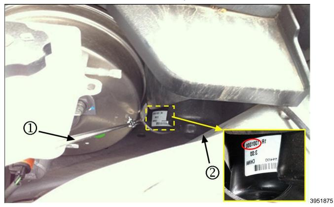
2. Reposition the water shield. Use a flashlight and inspection mirror (1) to view the
