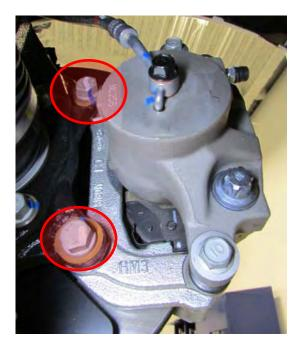
TSB #: 14-01-025 Page 4 of 6 5. Remove caliper assembly from axle assembly.
