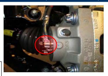
4. Remove caliper mounting bolts.
