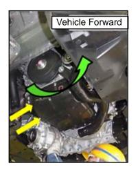
a. To create space for transfer assembly removal, roll the engine by pushing the oil pan towards the direction indicated by the yellow arrows. 12. Install the new transfer assembly P/N 3200A158. Please refer to the applicable service manual, Group 23C – Automatic Transaxle, Transfer Assembly (AWD) > Removal and Installation.
