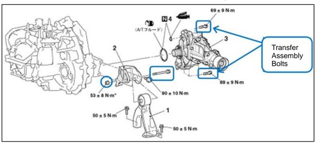
**NOTE:** Loosen the indicated transfer assembly bolts before removing the rear roll stopper.
