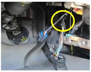
4. Connect the Late DRL Module to the connector. Do not fasten the module to the bracket at this time.
