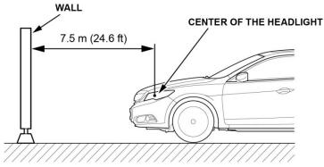
11. Measure the height of the headlight's center mark, then on the wall or screen, mark the same height of the headlights with masking tape in a straight line.
