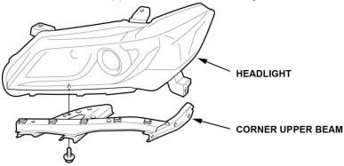
4. Install the corner upper beam to the new headlight and tighten the bolt to 9.3 N·m (6.9 lb-ft).
