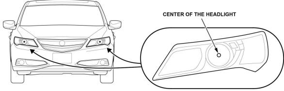
10. Park the vehicle on a level surface so that the center mark of the headlight is **7.5 m (24.6 ft)** away from a wall or screen.
