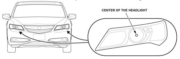
10. Park the vehicle on a level surface so that the center mark of the headlight is **7.5 m (24.6 ft)** away from a wall or screen.
