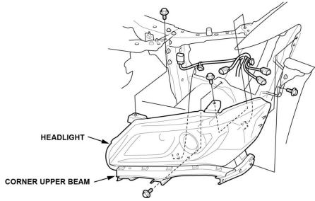
3. Remove the corner upper beam from the headlight.
