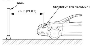
11. Measure the height of the headlight's center mark, then on the wall or screen, mark the same height of the headlights with masking tape in a straight line.
