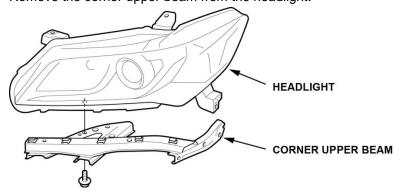
4. Install the corner upper beam to the new headlight and tighten the bolt to 9.3 N·m (6.9 lb-ft).
