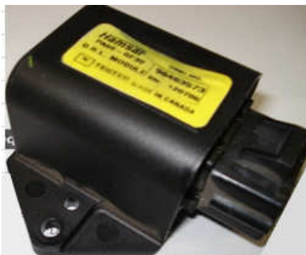
Heat Damaged DRL Module
