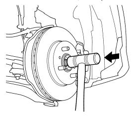
5. Pry the inboard joint from the differential using a pry bar. Remove the driveshaft assembly.
