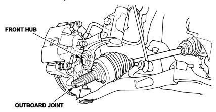
10. Wipe off any grease contamination from the ball joint tapered section and threads, then install the knuckle onto the lower arm. Be careful not to damage the ball joint boot. Wipe off the grease before tightening the castle nut at the ball joint. Torque the new castle nut to the lower torque setting 64-74 N·m (47-54 lb-ft), then tighten it only far enough to align the slot with the ball joint pin hole.
