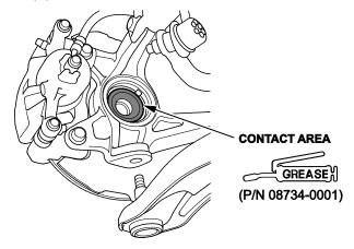
7. Clean the areas where the driveshaft contacts the differential thoroughly with solvent or brake cleaner, and dry them with compressed air.
