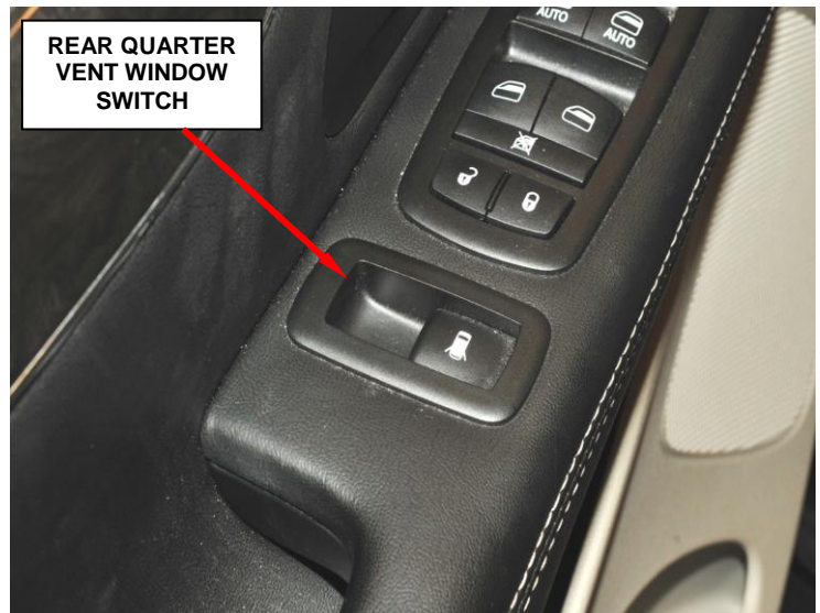
Figure 8 – Install New Rear Quarter Vent Window Switch
