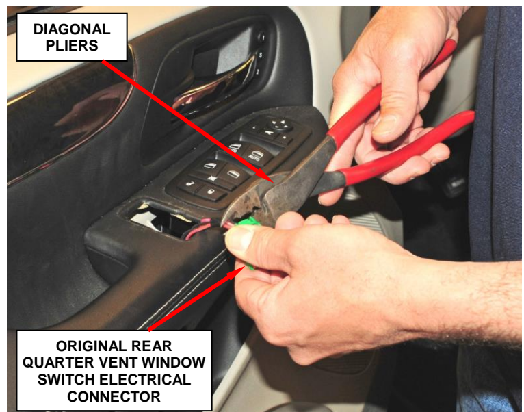
Figure 3 – Cut Off Damaged Connector
