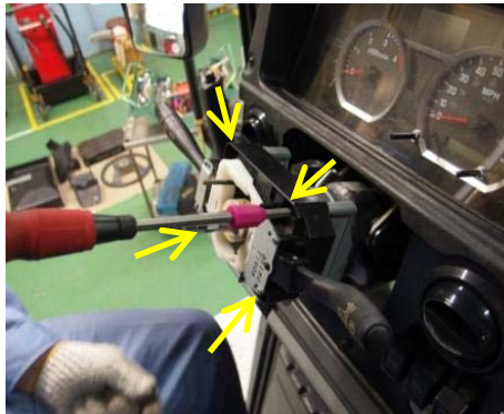
Figure 14 – Remove Combination Switch Assembly
