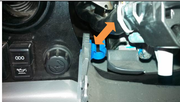
Figure 7 – Remove Harness from the Fixed Clip on the Steering Cowl
