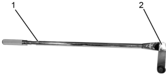
Figure 1. Torque Wrench 90 Degrees in Relation to Air Disc Caliper Wrench.
