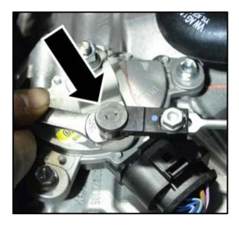
⇐ Pry the selector lever cable off the selector lever with the open end of an appropriate size wrench <arrow>.
