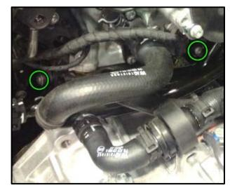
⇐ Reinstall and tighten the two mounting screws <circles> for the metal coolant lines.
