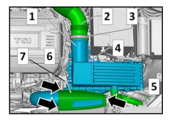
⇐ Unfasten the lower air intake tube by disengaging the clips <arrows>.
