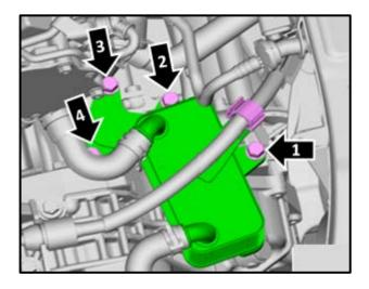
Remove the retaining bolts <arrows 1</p> through 4> from the ATF cooler.
