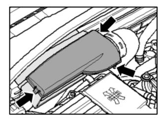
⇐ Reinstall the cover for the air intake hose and ensure the side clips <arrows> are properly engaged.
