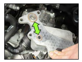
⇐ Gently lift the ATF cooler from the transmission and rotate the cooler toward the front of the vehicle to expose the O-rings <arrow>.
