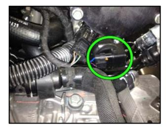
Remove the two retaining screws <circles> for the metal coolant lines.
