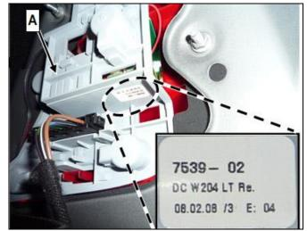
Figure 2 Example of bulb carrier that is: NOT OK (Production date up to and including 12.04.2012)
