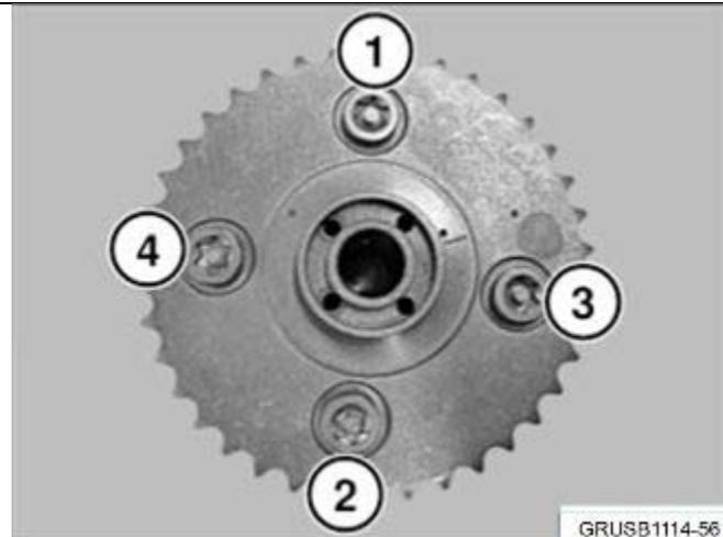
11. Replace and torque the aluminum bolts (1-4) one at a time.
