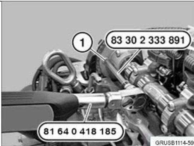
**7. IMPORTANT: The bolts require initial torque and angle torque. Observe the procedures in this step and the next step very carefully!**
