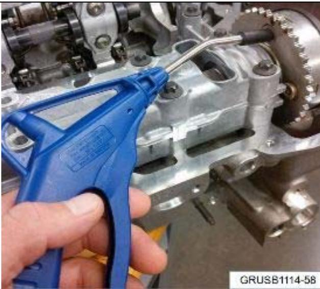
13. Clean the threads on the VANOS assembly using compressed air to remove the excessive oil.
