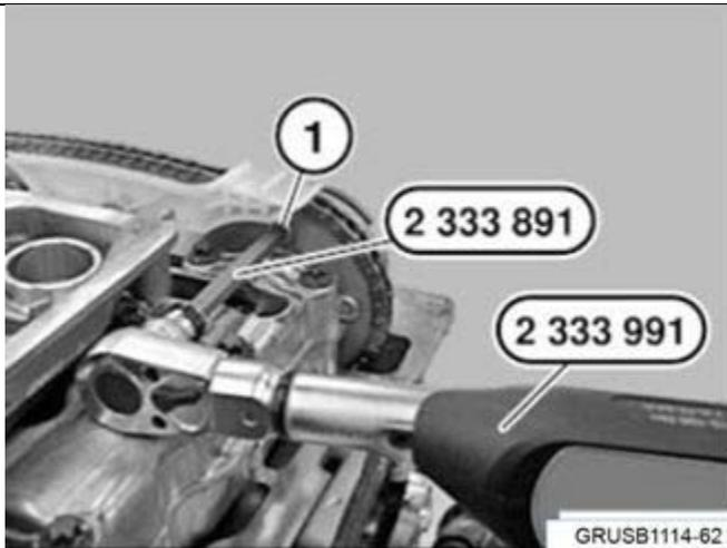
**14. IMPORTANT: The bolts require initial torque and angle torque. Observe the procedures in this step and the next step very carefully!**
