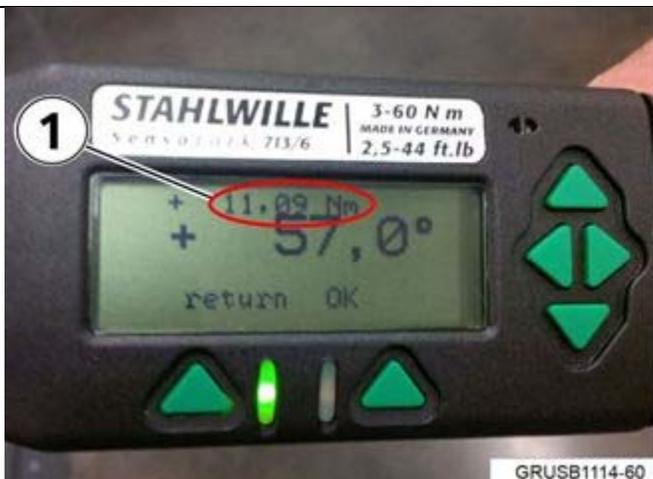
**8. While performing the angle torque, the digital screen on the torque wrench will display the current Nm meter value. This value should be between 8 Nm-14 Nm.**
