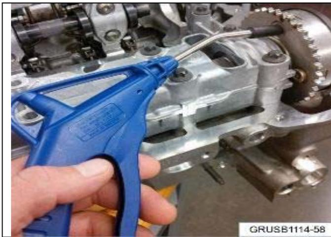
6. Clean the threads on the VANOS assembly using compressed air to remove the excessive oil.
