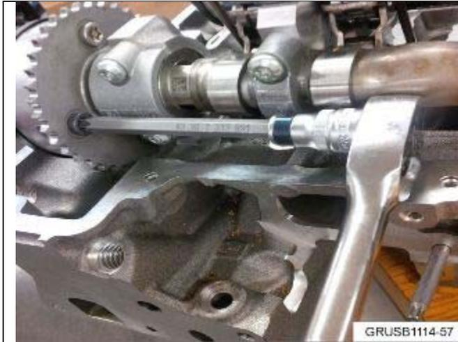
5. Turn the engine by hand, using a suitable tool on the crankshaft central bolt to align one of the bolts (1), as shown in the illustration.
