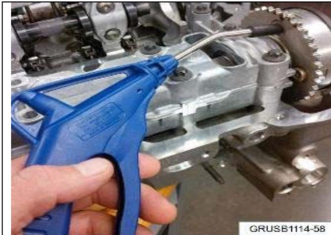
6. Clean the threads on the VANOS assembly using compressed air to remove the excess oil. The torque wrench results will be more consistent when cleaning the threads for more than 3 seconds.
