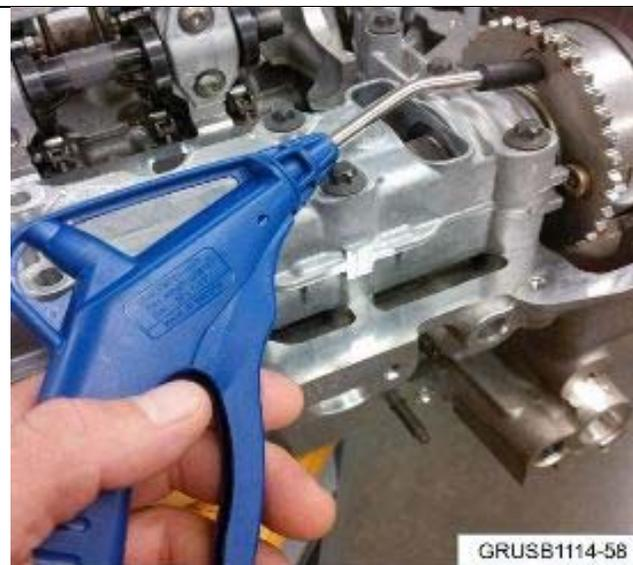
13. Clean the threads on the VANOS assembly using compressed air to remove the excess oil. The torque wrench results will be more consistent when cleaning the threads for more than 3 seconds.
