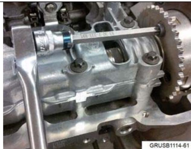
12. Turn the engine by hand using a suitable wrench on the crankshaft central bolt to align the bolt (1) as shown in the illustration.
