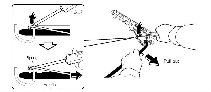
b) Lift the seat adjustment handle to release the lock and pull out the upper rail to access the adjustment handle lock plate.
