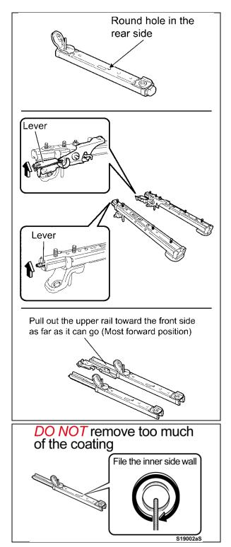
a) Pull the seat adjustment lever and adjust the upper rail so that it is in the forward most position.
