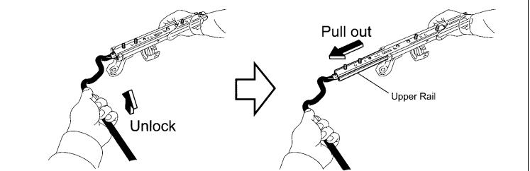
c) Using a flat tip screw driver, press the lock plate down and lightly turn the adjustment handle back and forth to remove it from the seat track.
