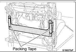
f) Check that gauge pins are properly seated and secure the gauge to the seat assembly using packing tape.
